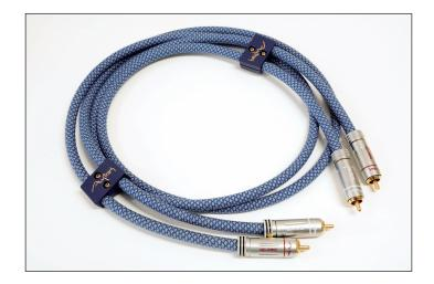
Using our direct plating technology, every single PC-triple C wire is plated by Gold and coated with urethane. Structurally stable 7 single wires are twisted to form one core wire. 2 core wires are covered by two different types of PVC and dual shielded. The braid is made of natural material. Specially selected material "ebonite" is adopted for the detachable clampers combining 2 cables, which absorb the vibration.
